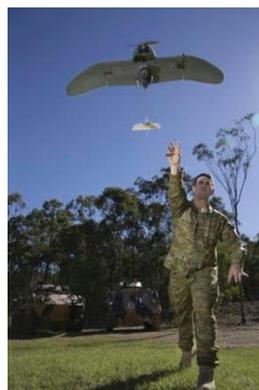
*Image: An AeroVironment Wasp AE being launched,*
